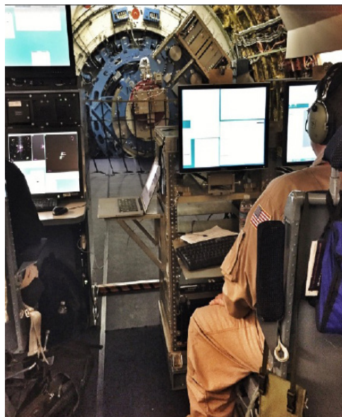
Inside SOFIA. The telescope is behind the blue structure in the tail section of the plane; the large box protruding from it is the liquid-He-cooled FORCAST camera used for our observations. On the left the telescope operator station. FORCAST is controlled from the station at the right.
