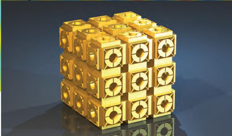
Dimensional isotropic design for optical negative index material suitable for direct laser writing application.
