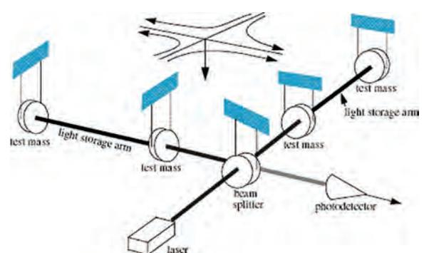
Diagram of a basic interferometer design. *Image courtesy of LIGO*
