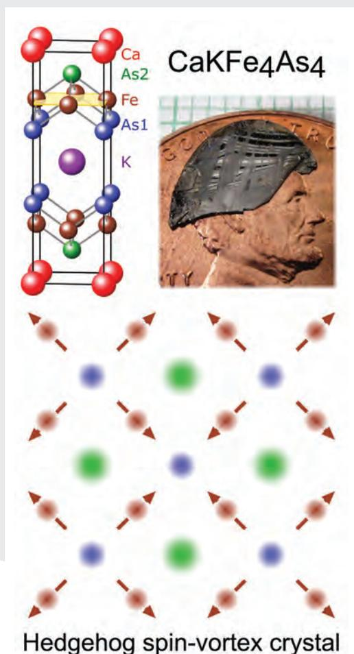
$\text{CaKFe}_4\text{As}_4$  unit cell, single crystal on a penny and magnetic structure inferred from diverse data sets.
